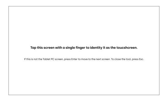
VERY IMPORTANT: If the message is displayed on the correct monitor then you can press the touchscreen with your finger as indicated on the message. However, if the message is displayed on the wrong display, you need to press enter until it is shown on the correct one
