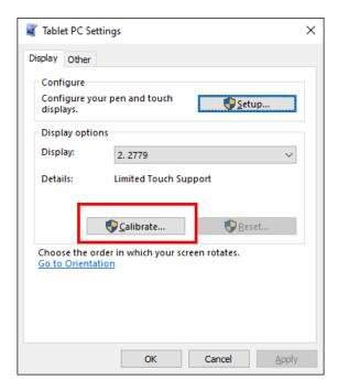
In the white screen, tap the crosshair each time that is appears on the screen, and do not change the resolution during this process.
